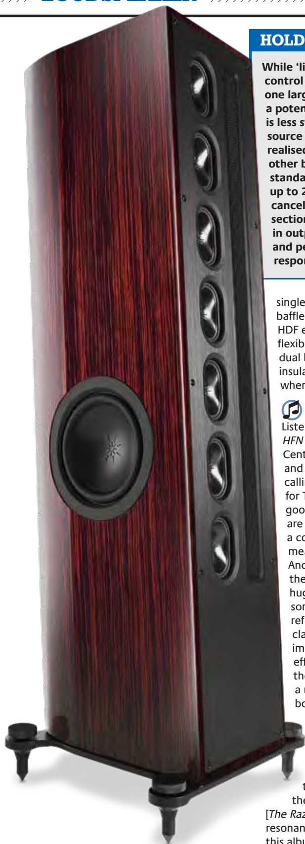
ABOVE: Two force-cancelling, long-throw 220mm 'StarStabiliser' bass units are mounted in opposition either side of the cabinet. Working up to 180Hz, they are reflex-loaded by a wide downward-firing port (hence the long spikes)
